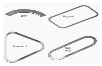
The rails are steel, induction hardened on the raceways, with the same section dimensions as straight FS..M rails. In the circuits the rails are joined together with alignment blocks that allow easy precise mounting.
